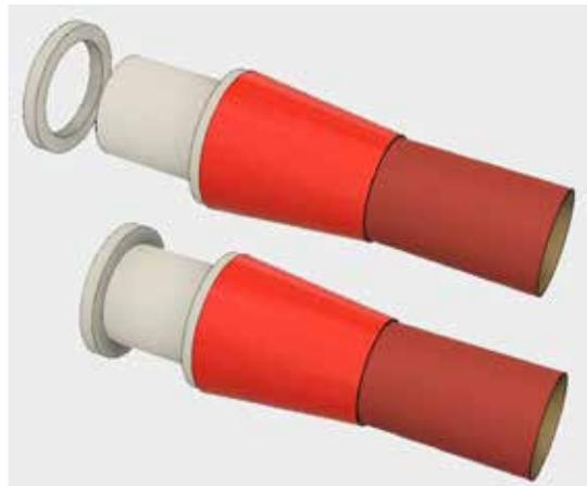
**Figure 18:** The forward centering ring is glued on the front end of the body tube.
