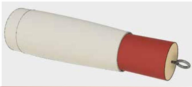
**Figure 11:** The completed transition that was made from a nose cone.
