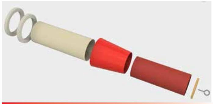
**Figure 20:** An exploded parts view of the paper transition section.
