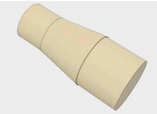
**Figure 8: A cast resin transition would be heavy, but easy to use.**
