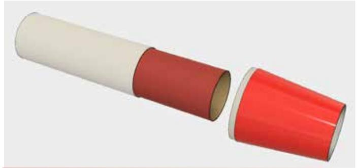
**Figure 17:** The transition is slid over the tube from the coupler side.
