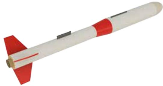
**Figure 2: The likely configuration of a TARC rocket that has a transition between the two tube diameters.**
