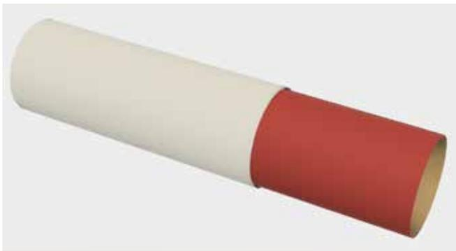
**Figure 15:** Glue the coupler into the body tube.
