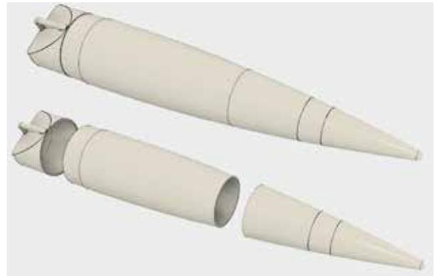
**Figure 9: Cut the base and the tip of the nose cone off.**
