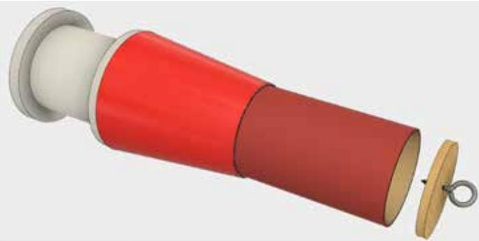
**Figure 19:** A bulkhead and screw eye are added to complete the transition.
