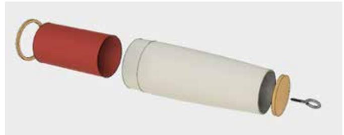
**Figure 13:** An exploded parts view of the transition made from a nose cone.
