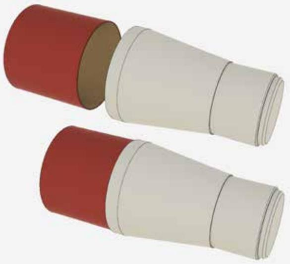
**Figure 21: A vacuum-formed transition with a paper coupler.**
