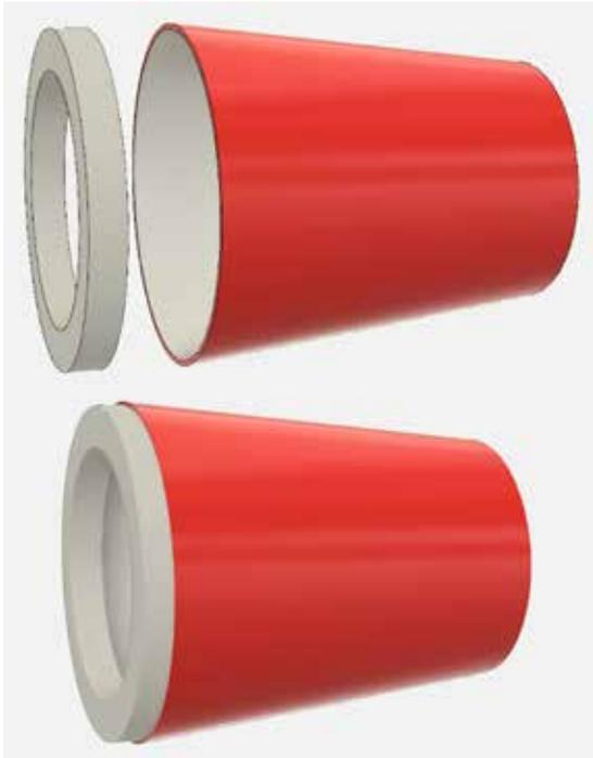
**Figure 16:** Glue the centering ring into the wide end of the transition. Half of the ring should extend out the end.
