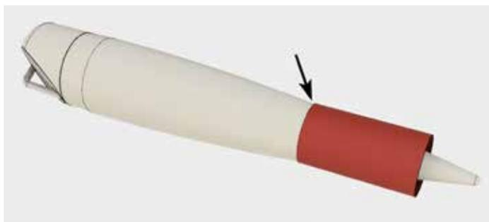
**Figure 10:** Slide a tube over the tip of the nose cone, and use the edge to draw a line around the perimeter. This will be the cutting line for removing the tip.
