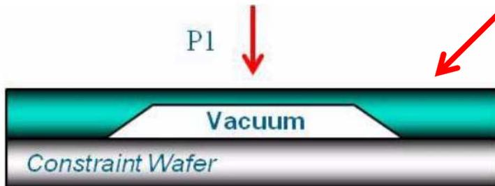
Cross section of absolute pressure-sensing element
